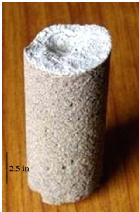
Fig. 2 Microbial sand plugging formed by Sporosarcina pasteurii (Bp M-3)
